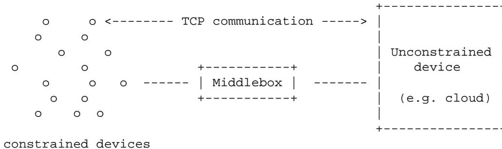
Figure 1: TCP communication between a constrained device and an unconstrained device, traversing a middlebox.
